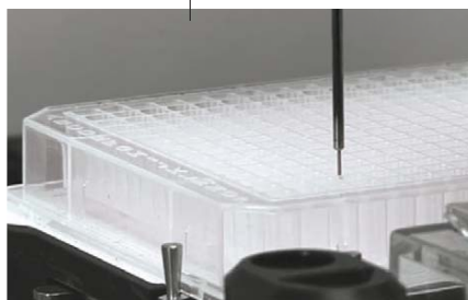
Minimal volume sampling capabilities, as little as 1 \mu L, conserve samples and reagent costs.
