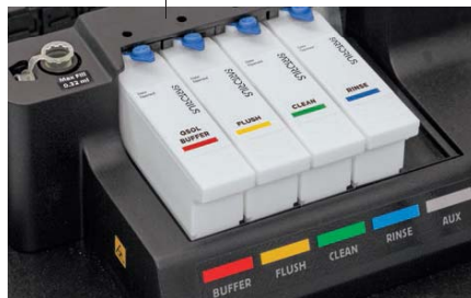
Extended run time on cartridges allows for unattended multiple plate processing. Liquid level detection and user-definable low-level warnings help ensure there are always enough reagents to complete planned runs.
